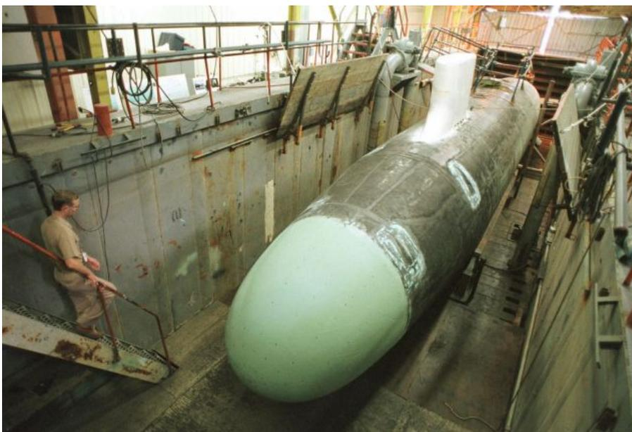
Both of these LSVs are built to run autonomously or semi autonomously and are guided using an advanced autopilot. This allows them to prowl the lake during tests without an umbilical harness attached, which greatly enhances test results during experiments where acoustic interference is a major issue.
