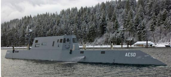
In 2005 the ARD got its first sub-scale surface vessel to operate and test, known as the Advanced Electric Ship Demonstrator (AESD), or by its sexier moniker "*Sea Jet*." *Sea Jet* is a 1/4 size functioning model of the Navy's *DDG-1000 Zumwalt Class* Destroyer that features a trapezoidal design and a unique [tumblehome hull](#). This hull configuration is highly controversial as analysts have noted that it may be less than stable in rough seas or during high-speed maneuvers.
