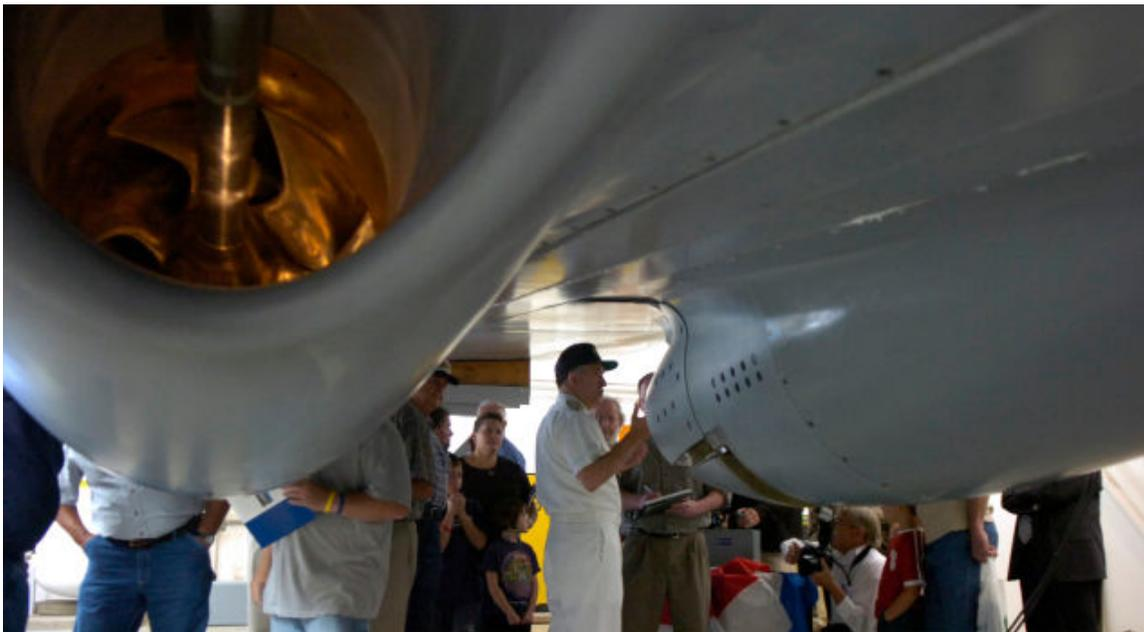
Like its submersible cousin, *Sea Jet* was built to be adapted to new missions and experiments without major overhaul. After all the test points were completed with the Rolls Royce propulsion concept, the ship was used to test General Dynamics "Rimjet" electro-magnetic podded drive system which could greatly change the way Surface Combatants' are propelled through the water in the future.
